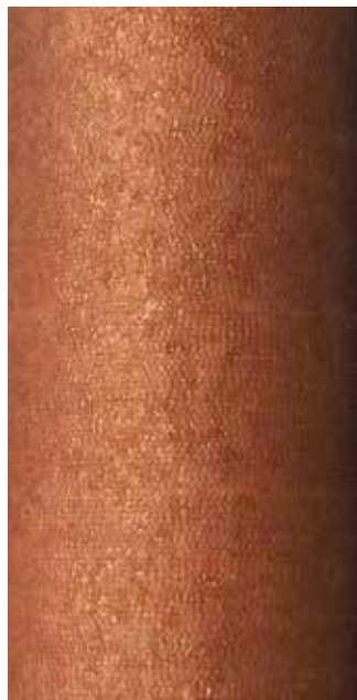
▶ Weathered Finish Self-protecting finish
